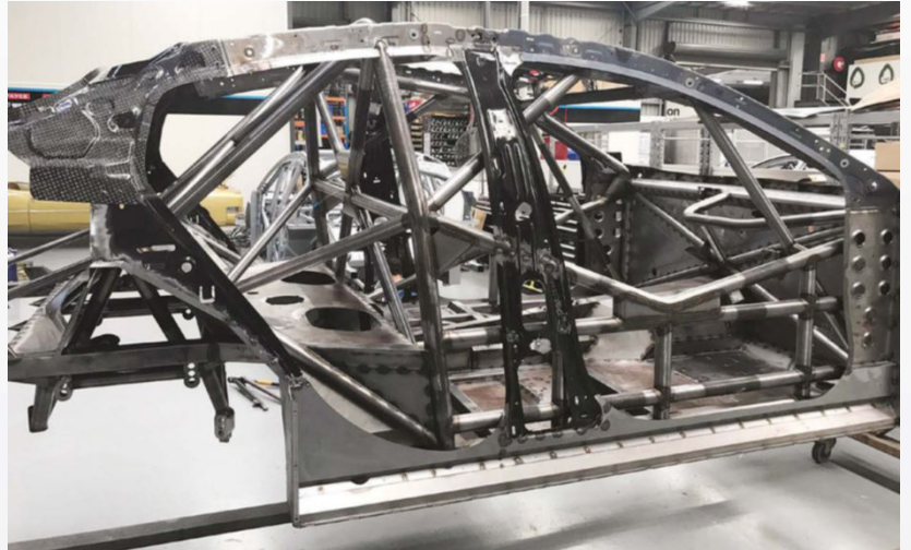
ABOVE & RIGHT. The control Supercars chassis remains the same between the Holden ZB and VF Commodore Supercars, along with the Ford FG X Falcon and Nissan Altima Supercars.
